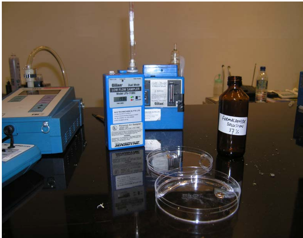
Air Sampling Equipment for Formaldehyde
