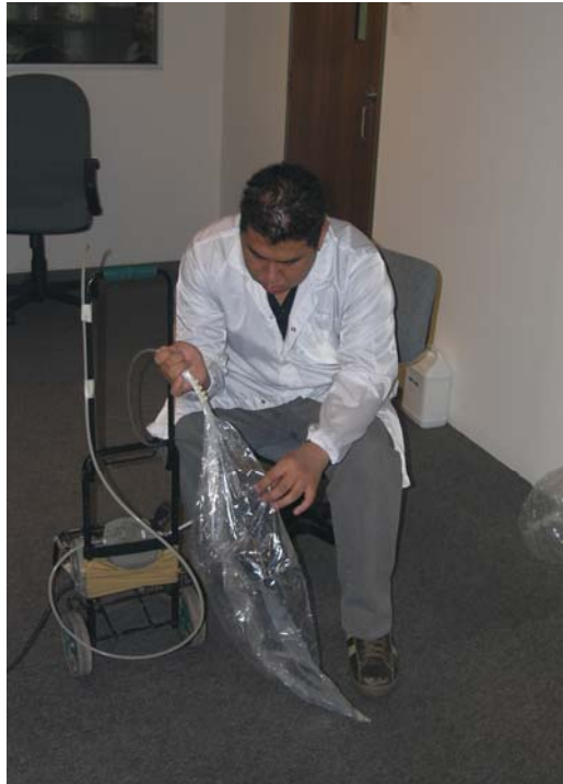
Odour sample was collected by using 40L capacity Nalophan bags with air sampling pump.
